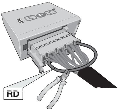
Pin 11 and Pin 2 disconnected
